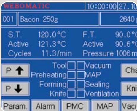
Colour touch screen with simple operating menu for process control and parameter setting of the PLC.
