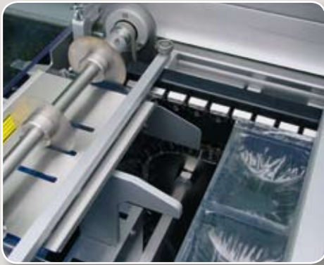
Longitudinal cutting with quick tension shaft.
