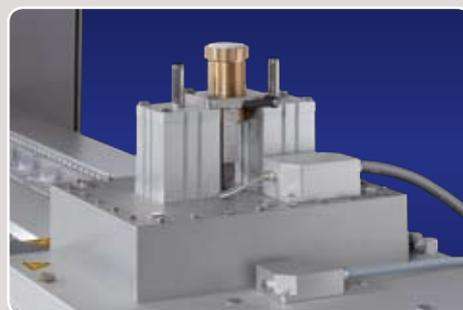
Forming die with sandwich-preheating and plug assist forming
