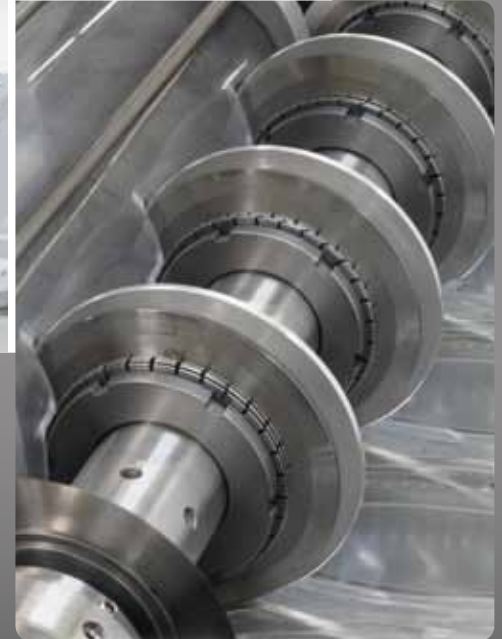
In order to prevent "cat nails", i. e. sharp-edged corners of the rigid film, apply the roll shear strip cutting in addition to the cross strip punch.
