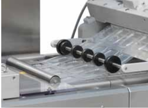
Top film forming: Useful for the creation of lids for reclosable packs.
