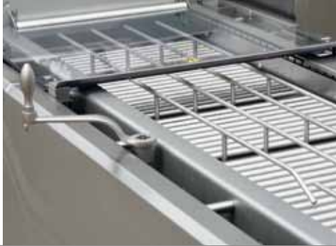
Employing a roller belt that is adjustable in height prevents heavy products from sagging.
