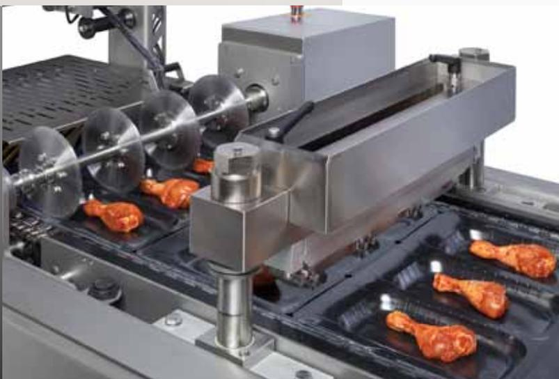
With a thermoformed skin pack, your product receives a skin-tight enclosure of a clear-transparent top film. This special skin film is being sealed onto the full surface of the bottom film without impairing the product. The result is a pack of excellent quality with enhanced food safety and the best possible product presentation – no matter if the product is presented hanging or lying at the point of sale.
